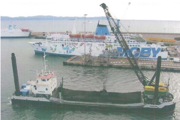
Figura 2c- Motonave splitte barge
