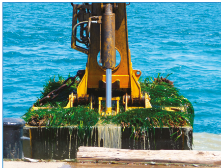
Figure 2 | Hydraulic clamshell bucket with explanted Posidonia oceanica clod.
